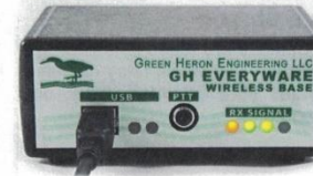
GH Everyware Remote with Radio Module and Connectors.
